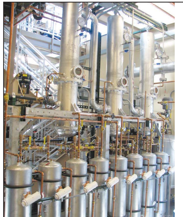
The completely refurbished Triple Effect, now fully instrumented and completely automated
